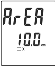
(4) Fig.4 Set Rectangle Duct X dimension.
