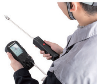
external pump gas detector
